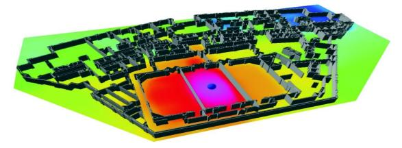
**CellTrace**<sup>™</sup> is a suite of software tools that addresses Radio Frequency (RF) planning, design, modeling, analysis and optimization of wireless communication systems within buildings, tunnels, stadiums and in campus environments.
